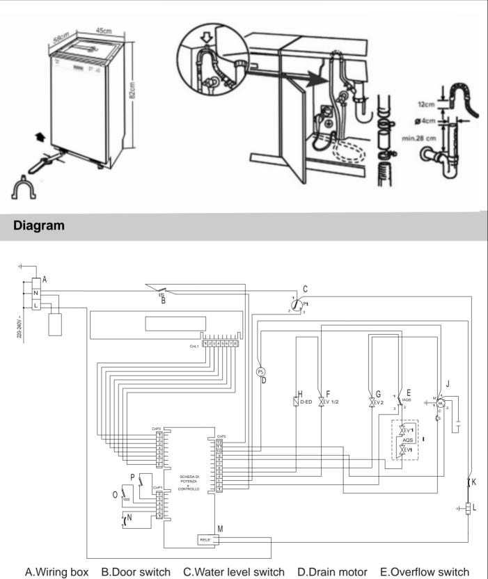
A.Wiring box B.Door switch C.Water level switch D.Drain motor E.Overflow switch F.Half wash switch G.Softer valve H.Dispenser valve I.Aquastop inlet valve J.Washing motor K.Temperature limiter L.Heater M.Relay N.Sensor temperature O.Salt missing switch P.Rinseing aid missing switch
